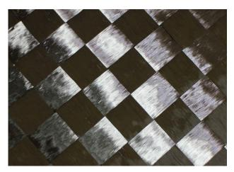
features carbon fiber fabric is widely used in various fields like aerospace, auto parts, sports equipment, building reinforcements, decorations, etc.
